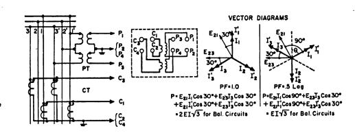
12. Metering: Watts on 3 phase 4 wire Transformers: 2 potential, 3 current trans. Instrument: 2-Element wattmeter Special Features: Preferably 8.66 ampere coils 1 imitations: Balanced voltages Cal. Watts =
