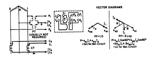
14. Metering: Watts on 2 phase 3 wire Transformers: 2 potential, 2 current trans. Instrument: 2-Element wattmeter Special Features: None Limitations: None, Standard connection Cal. Watts = Scale in watts P.T. ratio × C.T. ratio × 2
