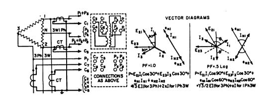
21. Metering. Watts on 3 phase 4 wire Transformers: 2 potential, 3 current trans. Instrument: 3-current, 2-potential wattmeter Special Features: None Limitations: Balanced voltages (bal. error small) Standard connection
