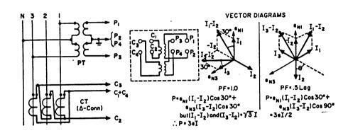
13. Metering: Watts on 3 wire 120 degrees (from 3 phase 4 wire) Transformers: 2 potential, 2 current trans. Instrument: 2-Element wattmeter Special Features: None Limitations: None. Standard connection
