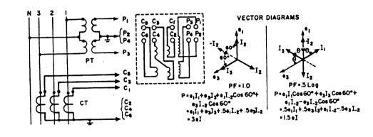
22. Metering: Watts on 3 phase 3 wire delta Transformers: 2 potential transformers 3 current transformers inside delta Instrument: 3-current, 2-potential wattmeter Special Features: None Limitations: Balanced voltages (bal. error
