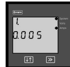
**System Amps Edit.** Pressing the ">> Next" key accepts the present value and returns the product to the measurement reading screens.
