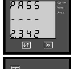
**New/Change Password.** Pressing the "↑ Adjust" key will scroll the value of the first digit from 0 through to 9. The value will change from 9 back to 0 if the "↑ Adjust" is pressed when 9 is displayed.
