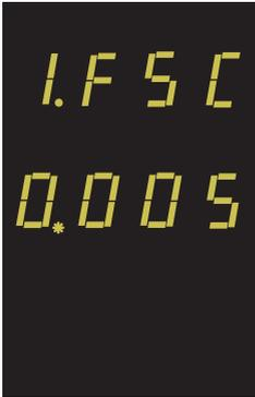
Pressing the "↑↓ Adjust" key will enter the "Full Scale Current Edit" mode. This will scroll the value of the most significant digit from 0 through to 4, the value will wrap from 4 round to 0. (0 to 9 for lesser significant digits)
