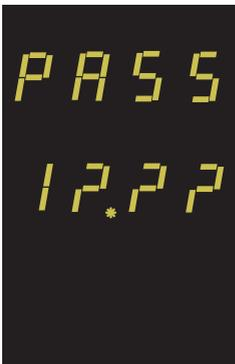
Enter Password, first digit entered, prompt for second digit. (\*decimal point indicates that this point will be flashing.)
