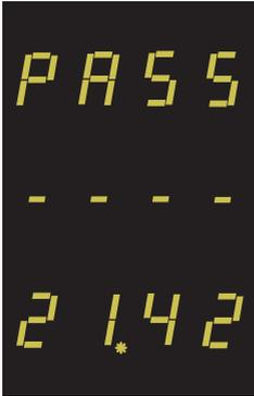
New/Change Password, first digit entered, prompting for second digit. (\*decimal point indicates that this will be flashing)
