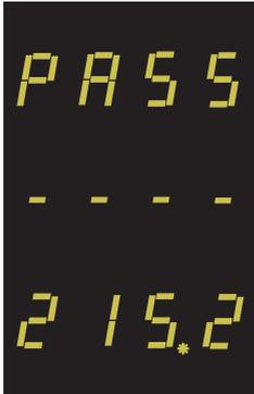
New/Change Password, second digit entered, prompting for third digit. (\*decimal point indicates that this will be flashing)
