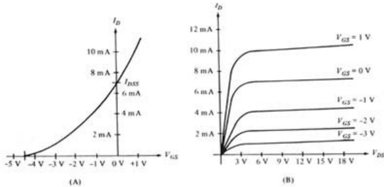
Figure (A), shows the transconductance,  $G_m$ , or effect of the gate voltage upon the drain to source current. Notice the gate-source voltage can be positive or negative. This would not be possible with a JFET. In figure (B), again notice the effect of increasing  $V_{gs}$  on  $I_{ds}$ ; notice also that for any given gate current, the drain-source voltage has little effect upon the drain current above 3 volts, since the MOSFET is in saturation.
