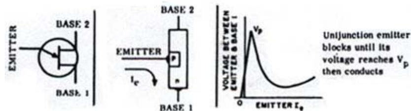
The emitter terminal does not inject current into the base region until its voltage reaches  $V_p$ . Once  $V_p$  is reached the base circuit conducts and a positive pulse appears at the B1 terminal and a negative pulse at B2. The UJT incorporates a negative resistance region, a low emitter current, and a high output pulse current at terminals B1 and B2, making it an ideal pulse trigger. A simple RC timer circuit using a UJT is shown below.
