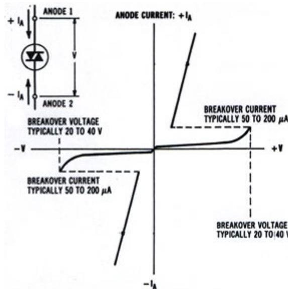
Although most diacs have symmetric switching voltages, asymmetric diacs are available. Typical diacs have a power dissipation ranging from 1/2 to 1 watt.
