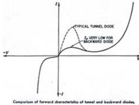
The reverse breakdown for tunnel diodes is very low, typically 200mV, and the TD conducts very heavily at the reverse breakdown voltage. Referring to the BD curve the back diode conducts to a lesser degree in a forward direction. It is the operation between these two points that makes the back diode important. Forward conduction begins at 300 mV (for germanium) and a voltage swing of only 500mV is required for full range operation.
