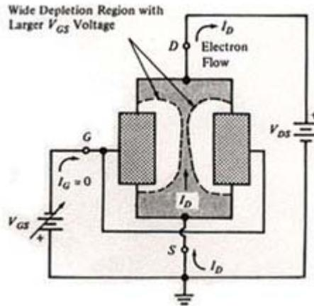
As a result, the the drain-source current is controlled by the gate voltage. Referring to the figure below, a typical JFET characteristic curve; notice the effect of the gate-source voltage on the drain-source current,  $I_{DS}$ . Notice the near linear relationship of drain current to drain voltage from zero to about one volt after that the JFET saturates. However, as the gate voltage is increased, the drain-source current is increased.
