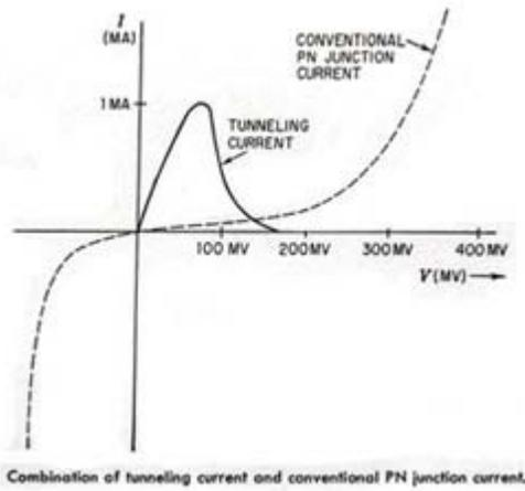
Resulting in a composite characteristic which is the tunnel diode characteristic curve.
