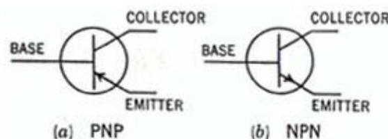
Note that the direction of the emitter arrow defines the type transistor. Biasing and power supply polarity are positive for NPN and negative for PNP transistors. The transistor is primarily used as an current amplifier. When a small current signal is applied to the base terminal, it is amplified in the collector circuit. This current amplification is referred to as  $H_{FE}$  or beta and equals  $I_c/I_b$ .
