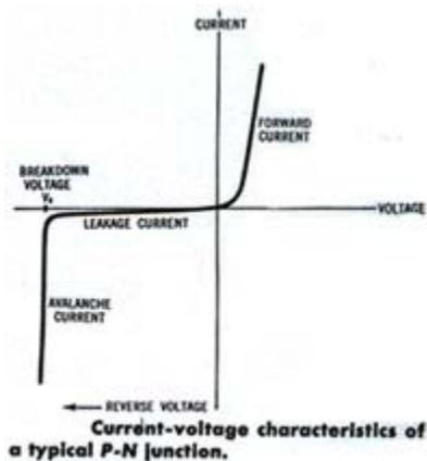
Notice that as the reverse voltage is increased the leakage current remains essentially constant until the breakdown voltage is reached where the current increases dramatically. This breakdown voltage is the zener voltage for zener diodes. While for the conventional rectifier or diode it is imperative to operate below this voltage; the zener diode is intended to operate at that voltage, and so finds its greatest application as a voltage regulator.
