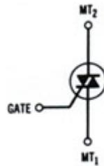
A triac operates in the same way as the SCR however it operates in both a forward and reverse direction. To get a quick understanding of its operation refer to its characteristic curve below and compare this to the SCR characteristic curve. It can be triggered into conduction by either a PLUS (+) or MINUS (-) gate signal.
