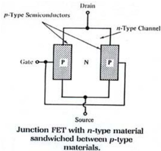
As with any reversed biased PN junction, a depletion region is formed which increases as the reverse gate voltage is increased. This depletion region, being devoid of majority carriers, reduces the channel drain-source current. *See figure below:*
