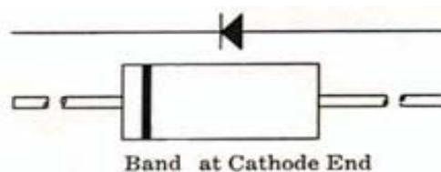
An ideal diode is like a light switch in your home. When the switch is closed, the circuit is completed; and the light turns on. When the switch is open, there is no current and the light is off.
