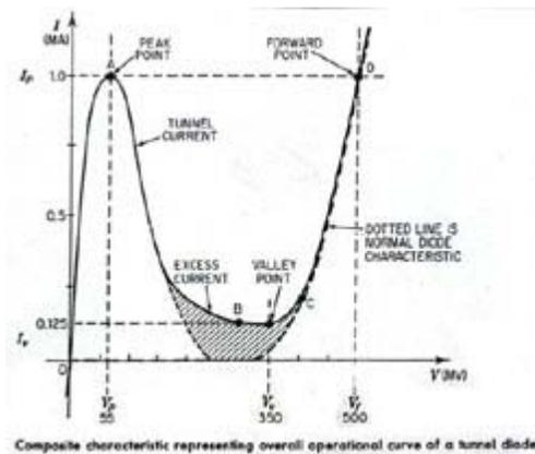
The negative resistance region (between points A and B) is the important characteristic for the tunnel diode. In this region, as the voltage is increased, the current decreases; just the opposite of a conventional diode. The most important specifications for the tunnel diode are the Peak Voltage ( $V_p$ ), Peak Current ( $I_p$ ), Valley Voltage ( $V_v$ ), and Valley Current ( $I_v$ ).
