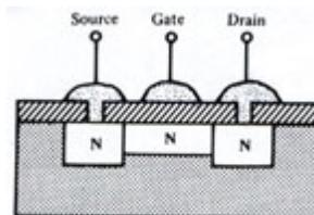
Notice that a positive gate voltage will induce a negative charge in the n-channel, enhancing the drain-source current,  $I_{ds}$ ; while a negative gate voltage will induce a depletion region in the n-channel, thereby reducing the drain-source current,  $I_{ds}$ . A MOSFET so constructed is a depletion/enhancement MOSFET. A typical n-channel MOSFET curve is shown below.
