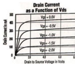
The figure of merit,  $G_{fs}$ , that is the ratio of drain-source current to gate voltage is the JFET transconductance.
