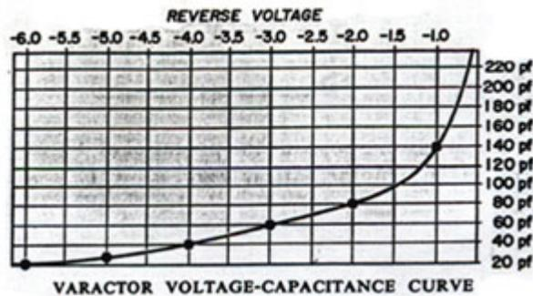
Notice the nonlinear increase in capacitance as the reverse voltage is decreased. This nonlinearity allows the varactor to be used also as a harmonic generator.
